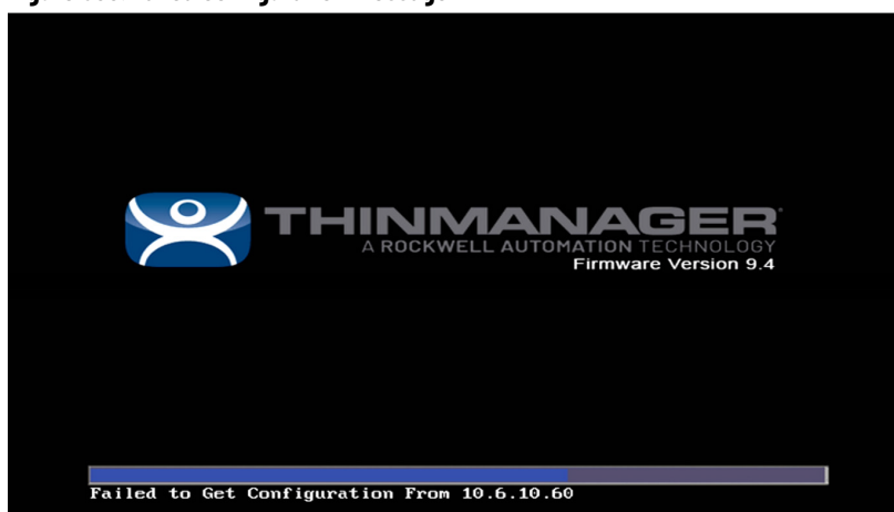
Figure 835. Failed configuration message
