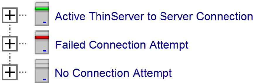
Figure 96. Remote desktop server status lights
