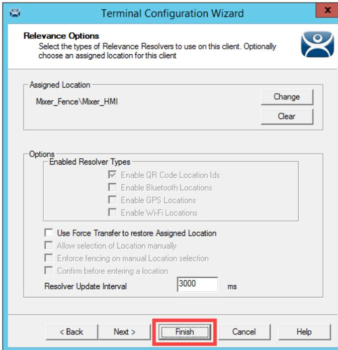
Notice the **Allow selection of Location manually** checkbox. With this checked, the **Terminal** to which this profile is assigned will be able to manually login to **Locations** that permit this action. In this scenario, if the **Enforce fencing on manual Location selection** is not checked, then the **Terminal** to which this profile is assigned will be able to login to any geo-fenced **Location** even when not within the geo-fence.
