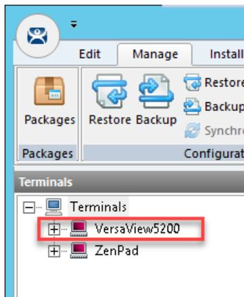
If you had a physical thin client and attempted to reboot it at this point, it would still be able to boot but not from the ThinManager installed on **RDS1**, instead **RDS2** would respond to the PXE request and boot the terminal. Unfortunately, we are unable to demonstrate this in the Cloud as the DHCP request from the virtual thin client does not make it to **RDS2** due to networking restrictions.
