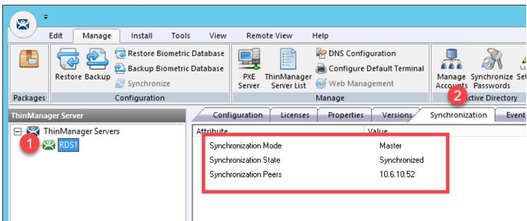
If the Synchronization State does not immediately show Synchronized, simply click on another tab, and return to the Synchronization tab to refresh its state.
