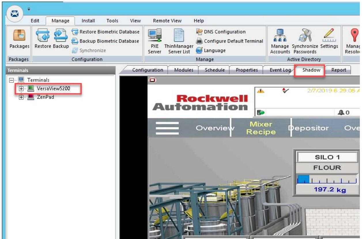
Terminal **shadowing** actually uses **TCP5900** for communication. This **outbound port** on **RDS1** was already enabled, but the **Terminal Monitor Connection** is first required before being able to establish a **shadow**.
