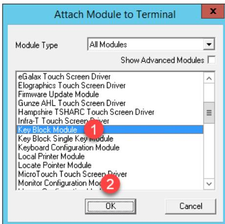
You may notice the **Key Block Single Key Module** and the **Keyboard Configuration Module** as well. The **Key Block Single Key Module** allows you to block specific keys, like CTRL-B, or any other combination, like ALT-S. The **Keyboard Configuration Module** provides the ability to set the initial state of the **Num Lock**, **Caps Lock**, etc., **Repeat Delay** and **Rate** as well as **Keyboard Layout** options.
