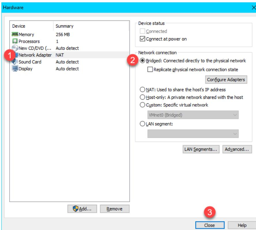
We have been using NAT for our virtual thin clients to this point in the lab. We will switch to Bridged in this section so we can see the desired network traffic in Wireshark. With that said, we will need to modify our PXE Server settings so that ThinManager will issue IP addresses for PXE requests.
