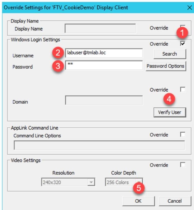
In addition to user credentials, the **Domain** can be overridden, along with the **AppLink Command Line** and **Video Settings**.
