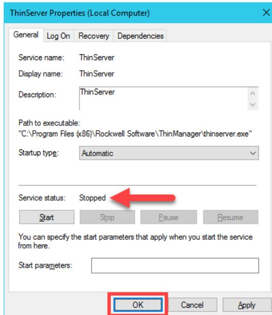
8. You have successfully disabled the **Secondary ThinManager Server**. The remaining lab sections can be completed with a single **ThinManager Server**. Close out of the **Computer Management** console on **RDS2**.
