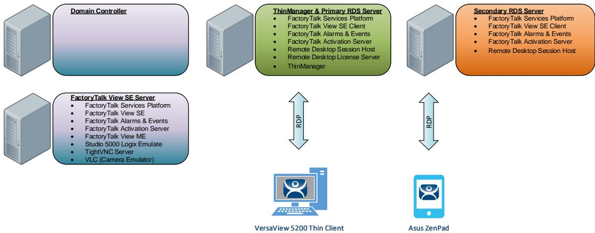
This lab utilizes 6 different VMWare images running in the Amazon Elastic Cloud (EC2) and will require you to perform tasks on RDS1, RDS2, DC and the two Virtual Thin Clients. An Active Directory domain was created named TMLAB.LOC. Each of the Windows-based images have been pre-joined to the domain. The four images are:
