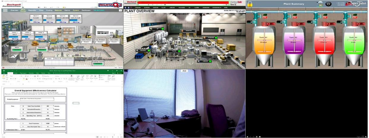
In addition to using **Tile Mode** to switch between the **Display Clients**, the **Display Client Selector** at the top of the terminal can be used. To use the **Display Client Selector**, click and hold the selector to expand the menu. While still holding the mouse button, point to the desired **Display Client** and release the mouse button to select it. You can also return to **Tile Mode** from the **Display Client Selector**.
